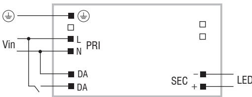
PUSH SWITCH diagram - Collegamento PUSH SWITCH
